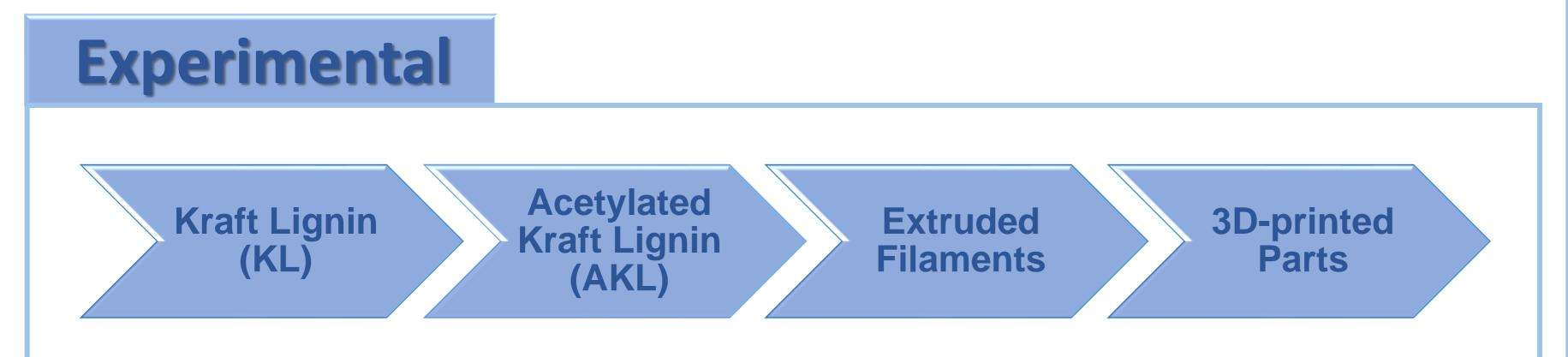
**Lignin Modification:** the acetylation was carried out at a ratio of 1 g KL:1 mL acetic anhydride:1 mL pyridine, for 24 h at room temperature.
